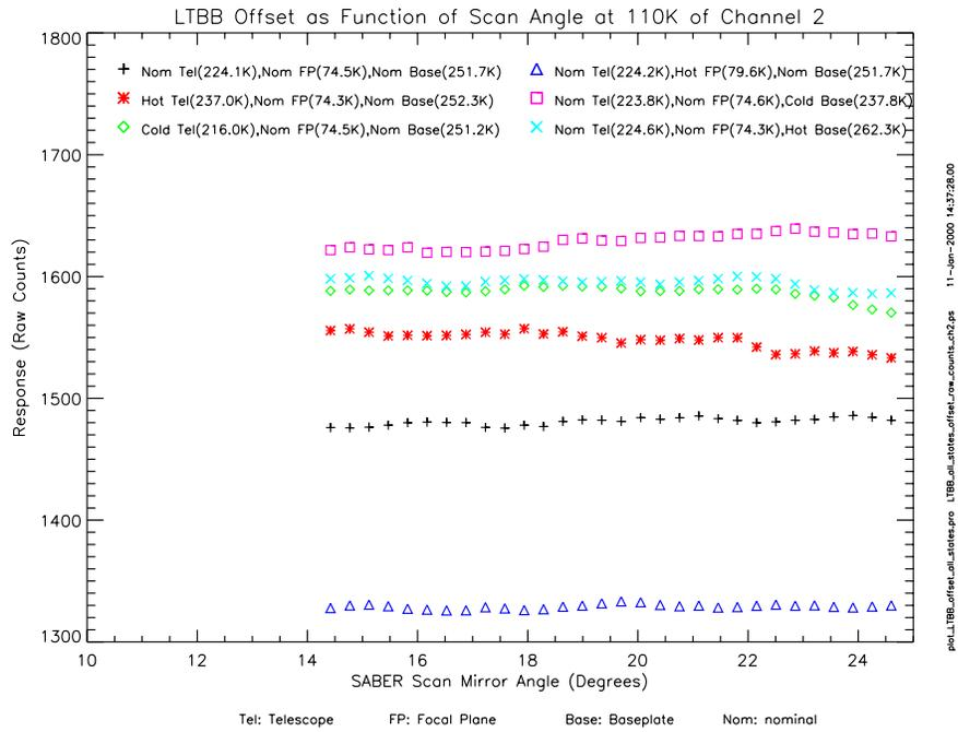
Figure 13. Relative offset versus scan angle for channel 2
