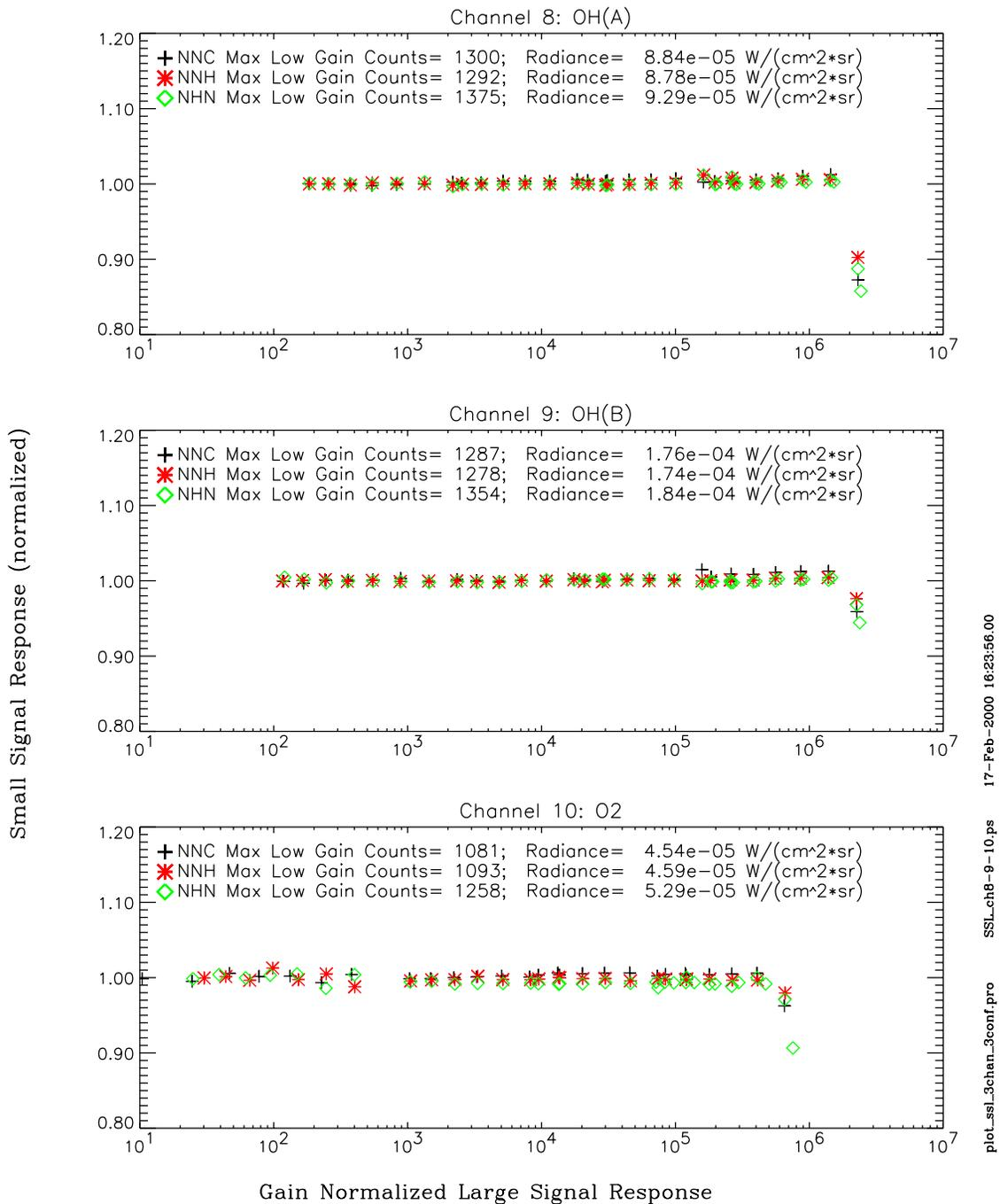
Small signal response was normalized between ND filter settings by calculating the ratio of overlapping two points between adjacent ND settings except channel 8 NHN and NNH ND0 and ND1.
