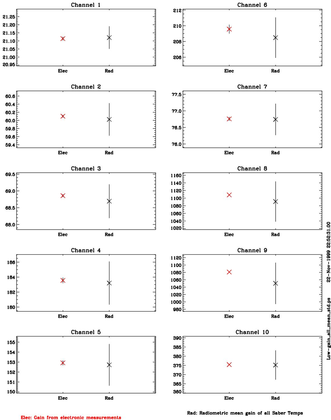
Figure 36. Comparison of medium gain values determined from electronic bench measurements with values determined from radiometric measurements
