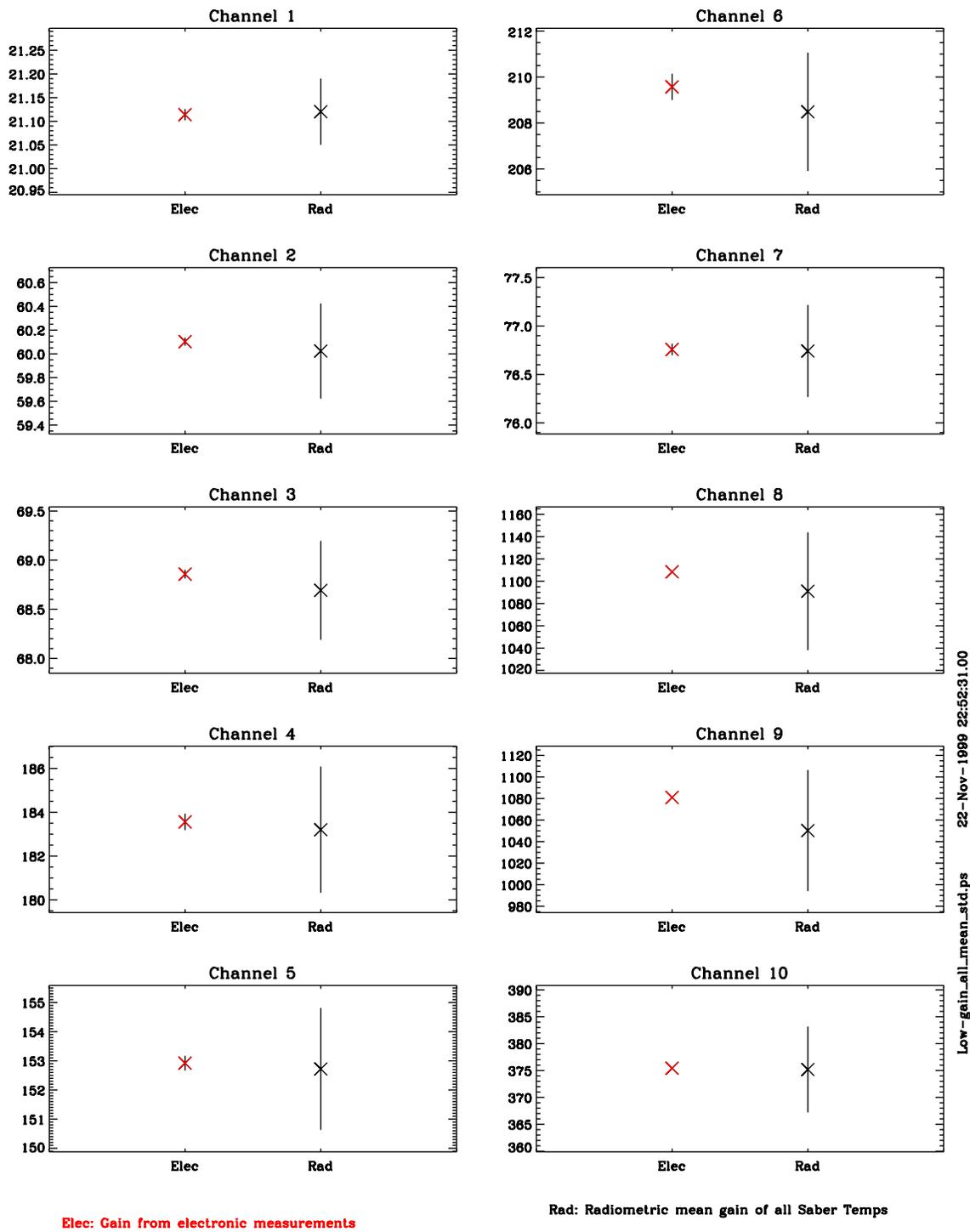
**Figure 35. Comparison of low gain values determined from electronic bench measurements with values determined from radiometric measurements**
