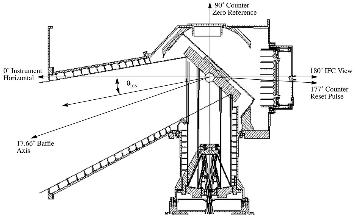
**Figure 99. Scanner mechanism**
