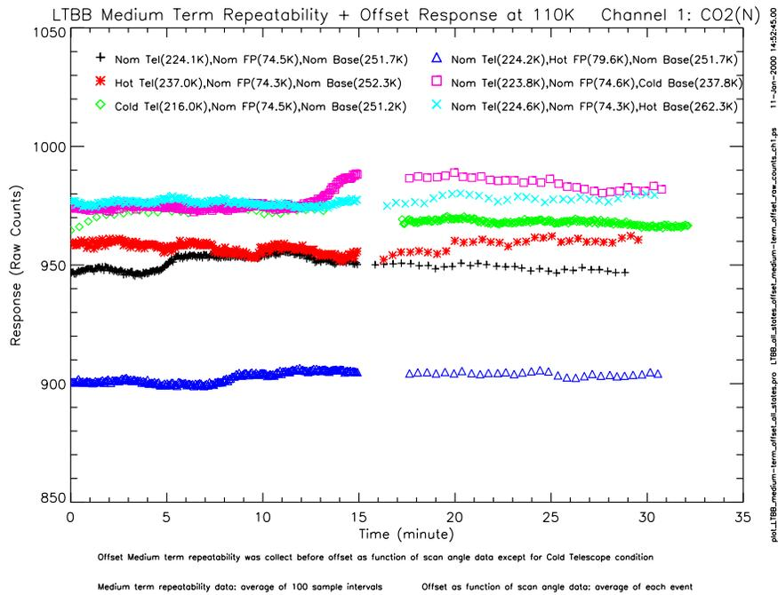
Figure 22. Relative offset time series for channel 1
