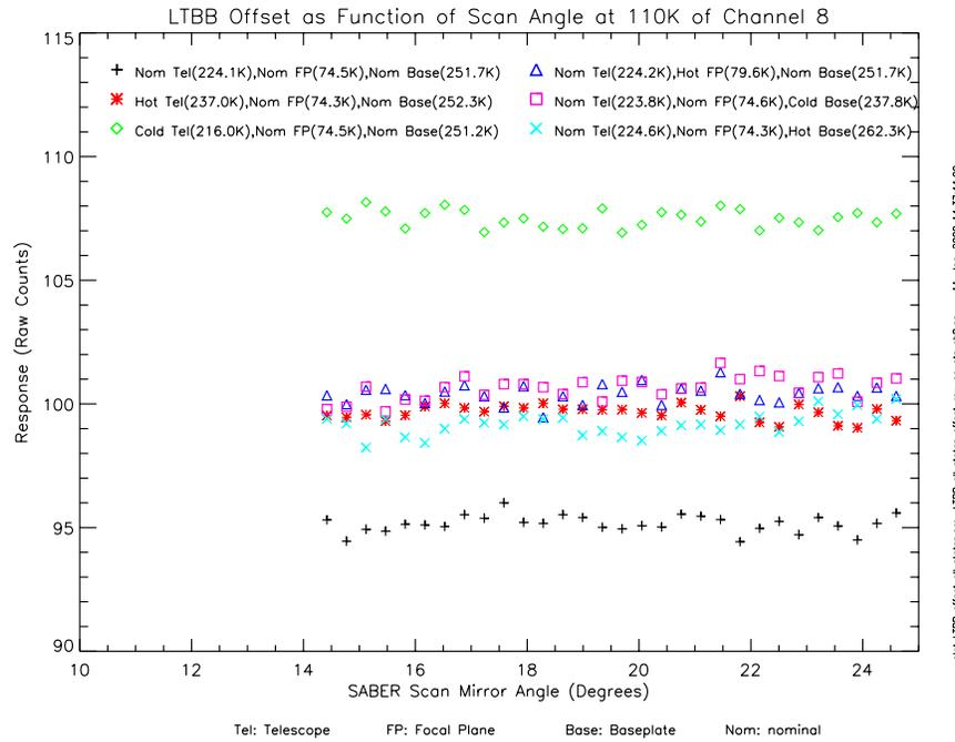
Figure 19. Relative offset versus scan angle for channel 8
