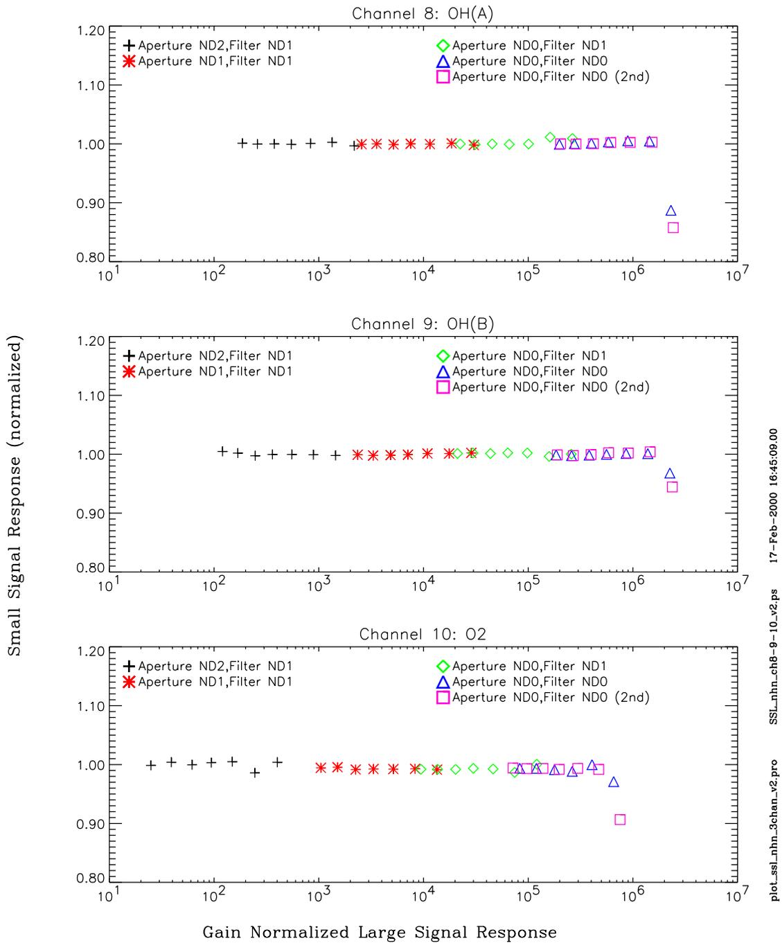
Small signal response was normalized between ND filter settings by calculating the ratio of overlapping two points between adjacent ND settings except ch8(ND0-ND1).
