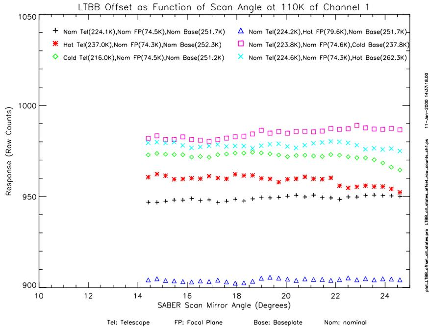
**Figure 12. Relative offset versus scan angle for channel 1**
