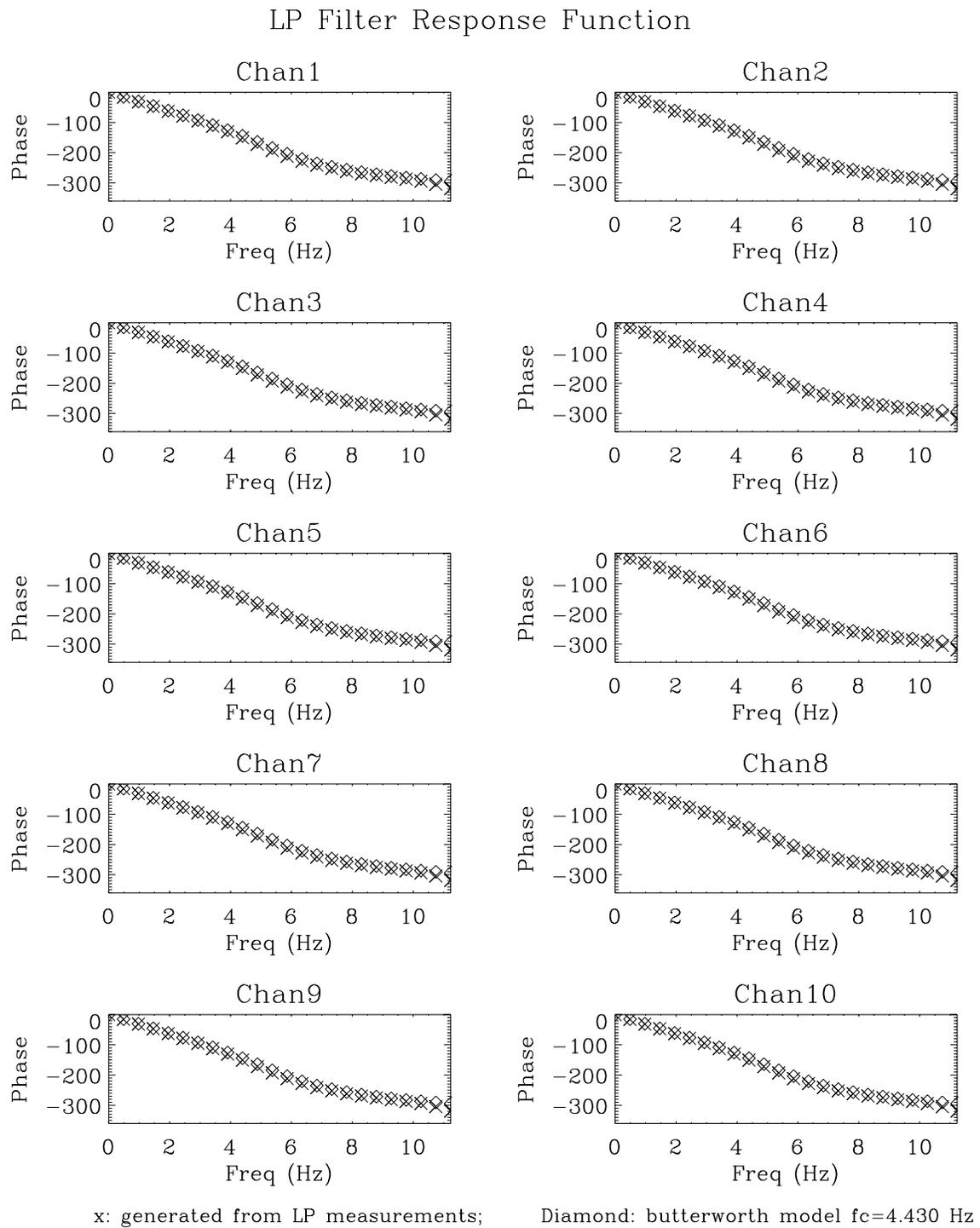
**Figure 103. Low-pass filter phase response**
