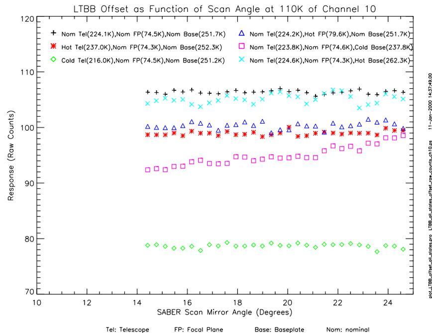
**Figure 21. Relative offset versus scan angle for channel 10**
