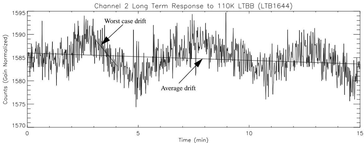
**Figure 32. Example offset drift for channel 2**
