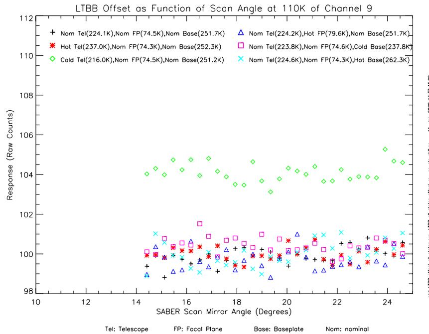
Figure 20. Relative offset versus scan angle for channel 9
