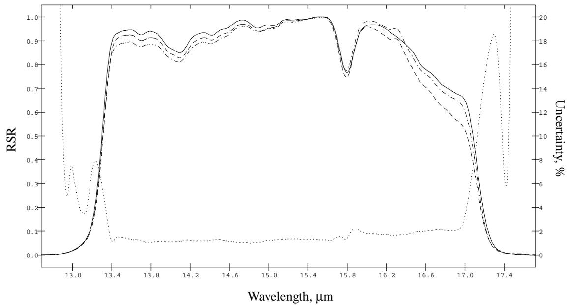
**Figure 69. SABER channel 3 RSR**
