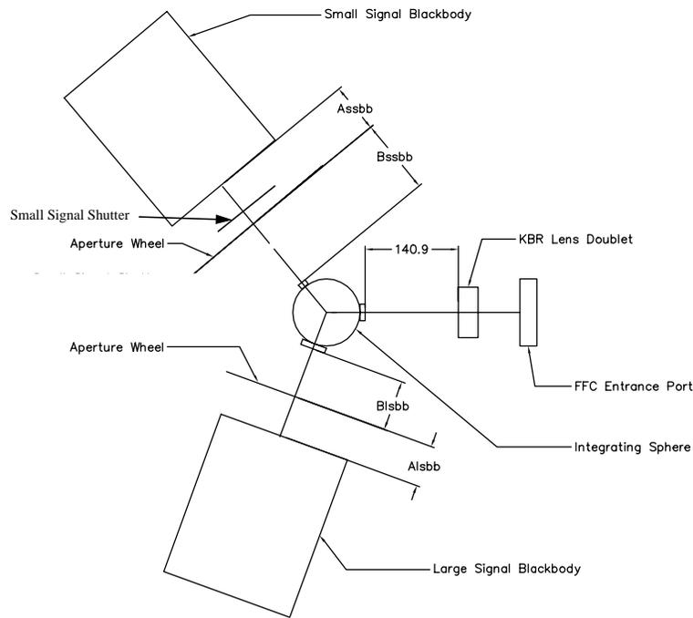
**Figure 48. Small-signal linearity test configuration for channels 8, 9, and 10**
