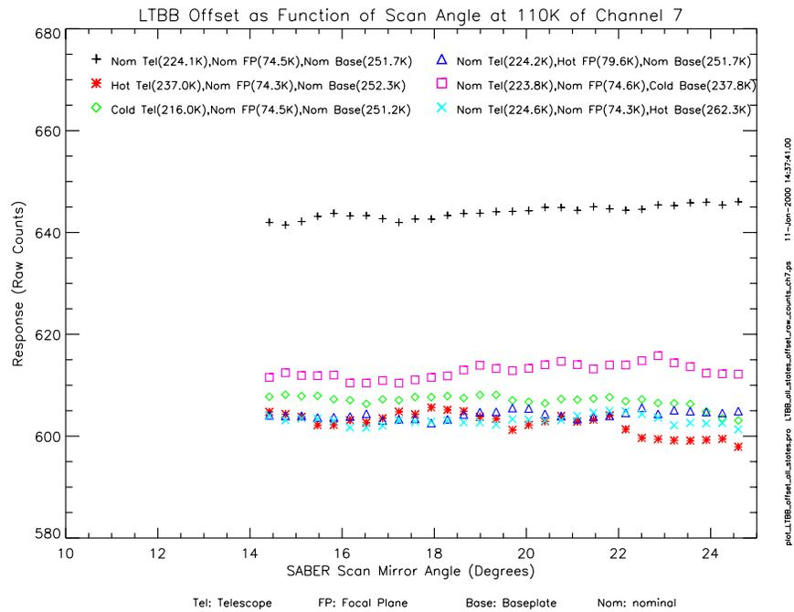
Figure 18. Relative offset versus scan angle for channel 7
