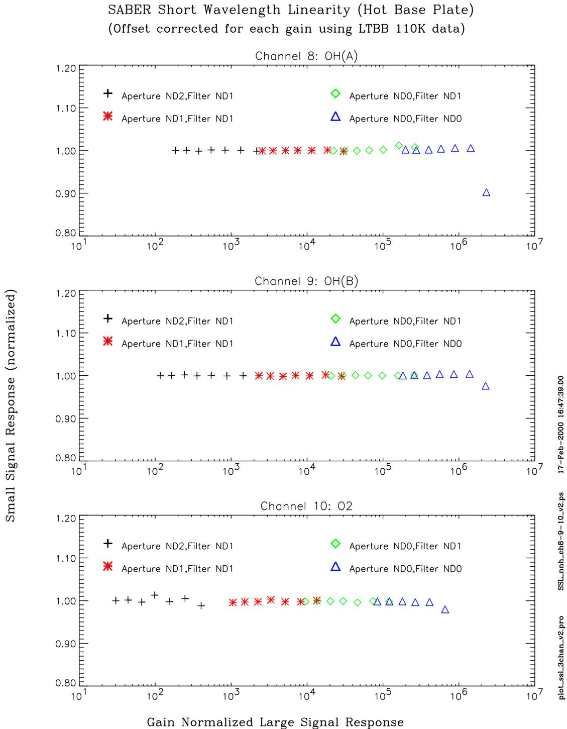
Small signal response was normalized between ND filter settings by calculating the ratio of overlapping two points between adjacent ND settings except ch8(ND0-ND1).
