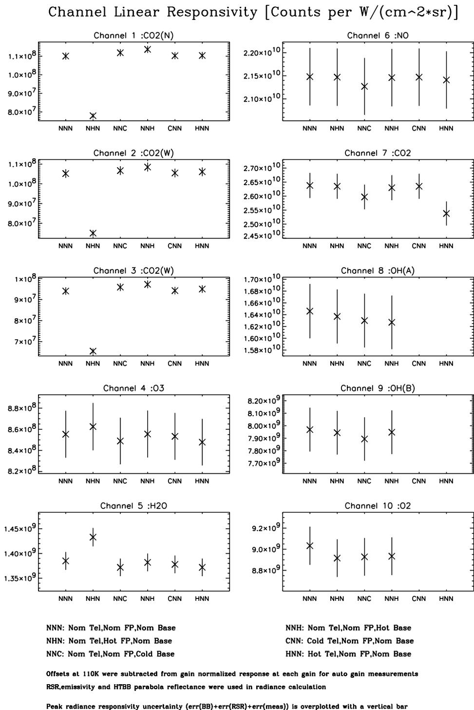
**Figure 47. Channel responsivity for each SABER temperature state**
