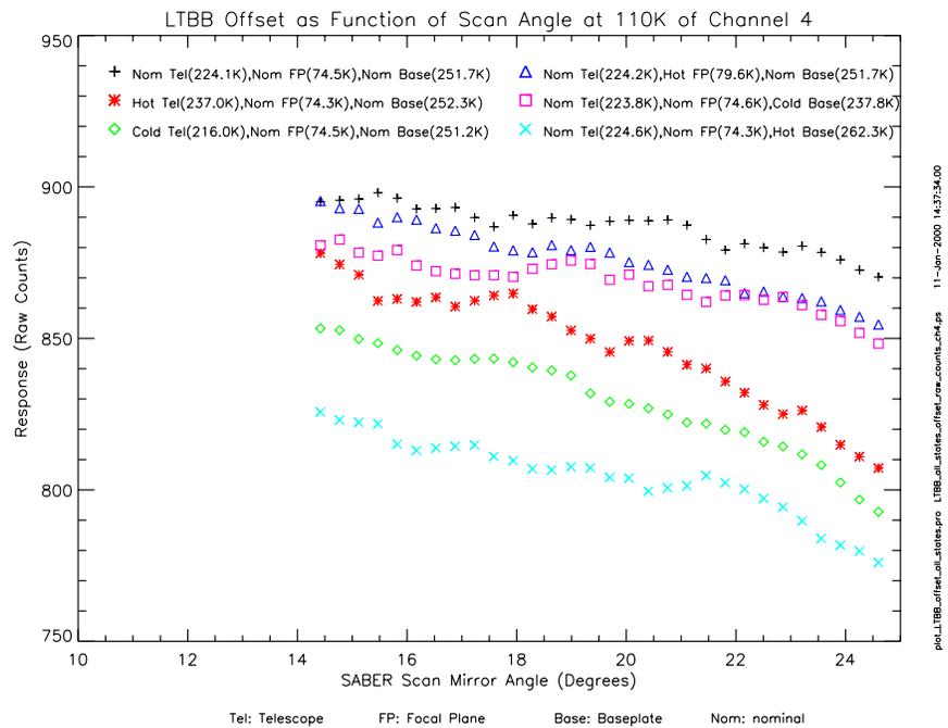
Figure 15. Relative offset versus scan angle for channel 4
