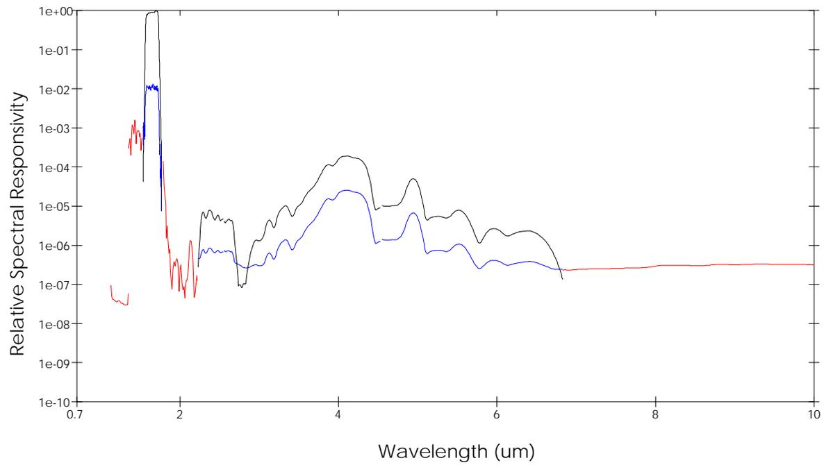
**Figure 86. Out-of-band RSR - channel 9**
