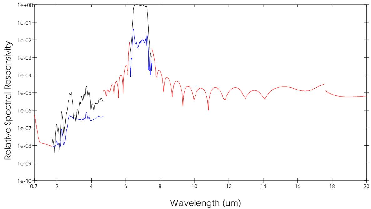
**Figure 82. Out-of-band RSR - channel 5**
