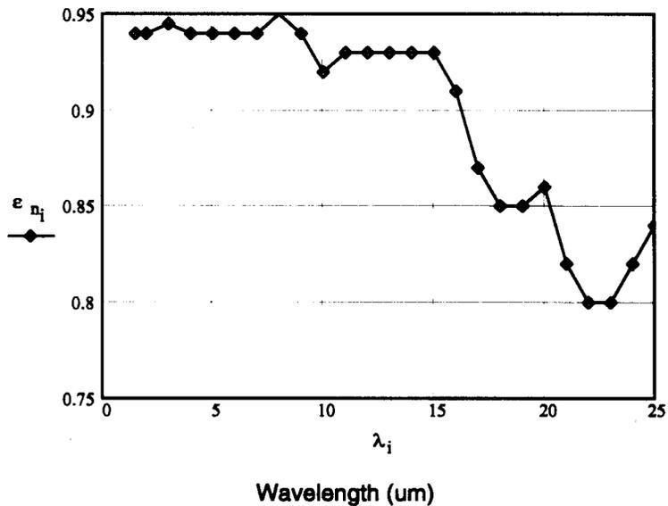
Estimated hemispherical emissivity based on Z306 type reflectance variation where hemispherical reflectance is double the normal reflectance.
