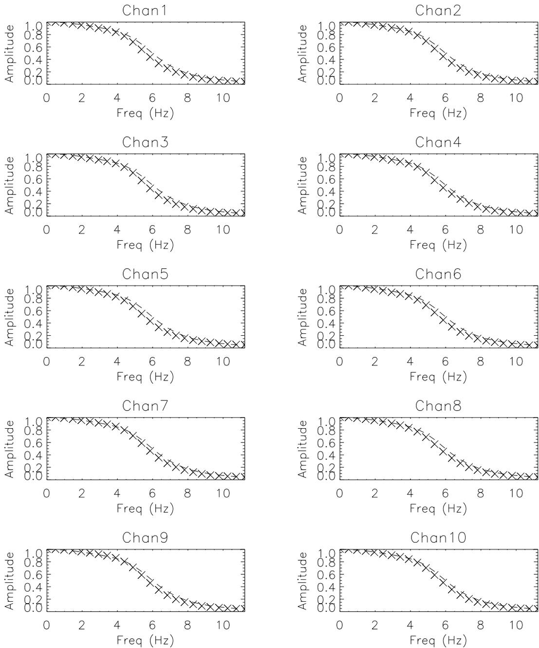
x: generated from LP measurements;      Dashed: butterworth model fc=4.430 Hz
